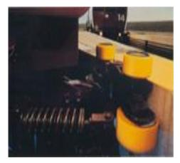
**Material handling equipment wheels** have a core of Cast Iron & nylon wheels, which is bonded with Polyurethane (PU) for Extra Life; PU is wear and tear resistant and also a scratch free material. It provides about 8 to 10 times the life of a rubber and nylon. PU Wheels can be designed to handle any load under the widest possible environmental conditions. Industrial wheels can be designed for high cut and wear resistance and also to provide
